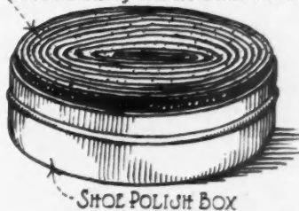
A Shoe Polish Box Containing a Coil of Oil Soaked Felt for Oiling Saws.
