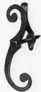
No. 1685 1/2 With non-rattling device. Blind fits between the "S" hook and the phosphor bronze spring. Tension holds the blind rigid and prevents rattling.
