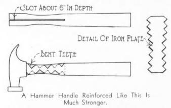
into the saw cut with the teeth only protruding. The teeth in the plate can be sawed out. I then insert the plate in the slot and bend the teeth around the handle, as shown. The teeth are bent alternately, first to one side, then to the other. This makes the handle about four times as strong and will save the inconvenience of a broken handle.
