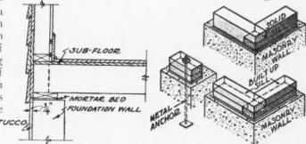
Figure 16.—Showing the posi- Figure 17.—Framing of sills at tion of the sill on wall when the wall is to be stuccoed.
