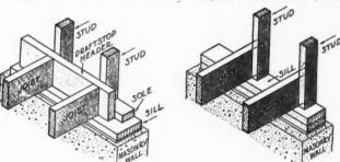
Figure 7.—T sill construc-
