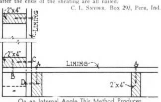
On an Internal Angle This Method Produces a Good Job of Framing.
