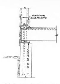
FIGURE 19.—Showing method suggested for anchoring where conditions are extreme. Bolt may be replaced by hooked rod threaded at one end.
