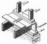
Figure 9.—Box-sill construction for western framing.
