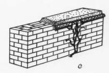
Figure 15.—Methods of preventing damage by termites or white ants; "a" shows a foundation wall of hollow tile surfaced with stucco; note the metal termite shield; the top of the wall is capped with slate and concrete; "b" shows a concrete wall with termite shields on the wall and around the pipes; "c" shows brick wall with termite shield capped with concrete. (Courtesy of the Bureau of Entomology.)
