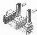
Figure 10.—Sill construction for braced framing.
