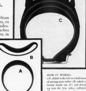
(A) Added to the tube is a half moon of springy gum rubber (B) which is turned inside out (C) and forced up into the tire, when inflated. This gum rubber quickly springs together preventing even a nail-hole from causing leakage of air.
