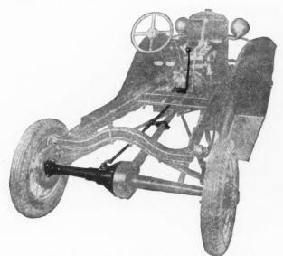
This Axle Unit Gives Any Ford Car the Advantages of a Four-Speed Transmission.
