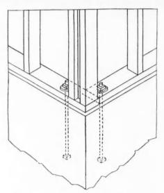
FIGURE 20.—Method of butting sills at the corners. Note the bolts near the corners.
