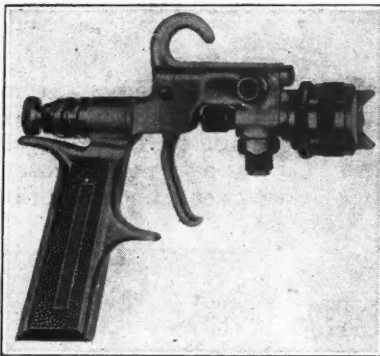
A variety of kinds of synthetic lacquers can be handled by this new spray gun and head attachments
