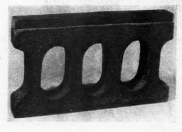
Light weight concrete from expanded slag aggregate.
