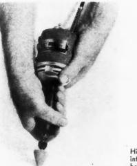
High speed grinder gets into irregularly shaped holes and hard to reach places.
