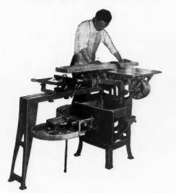
Cross cutting with the Electric Carpenter—band saw lowered to borizontal position. Seven machines in one:—Lathe, Shaper, Jointer, Band Saw, Mortiser, Saw Table, Speed Spindle.
