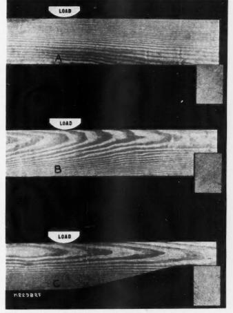
TESTS SHOW THAT JOIST B, notched to one-half depth, is good for a load only one-fourth of that carried by the unnotched joist A. Joist C, with the shoulder of the notch cut away, will carry twice the load of B or one-half that of A.
