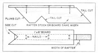
Plumb and side cuts can be marked without moving.
