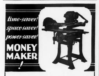
This remarkable machine cuts costs as quickly and as surely as it cuts wood! Does the work of five ordinary machines—eighteen different everyday jobs—faster and at less cost! Cross-cut saw, rip saw, jointer, shaper and router—five machines in one . . . at the cost of one. Ball-bearing throughout. Write for full particulars.
