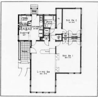
THE floor plan measuring about 34 feet wide by 42 feet deep gives  $4\frac{1}{2}$  large well lighted rooms. It is a popular "apartment lay-out."
