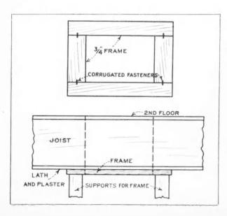
Rig at left is used to get clean cut hole in plaster.
