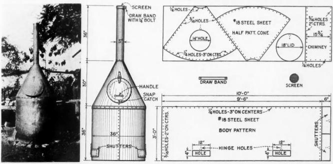
Home made incinerator cost only \$14 to build and takes care of refuse from 18 families. Metal pattern for parts is given.
