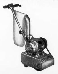
work. The steel wool drum is becoming more important, due to the popularity of penetration or steel finish floor treatment. A 1 H.P. 110 volt
