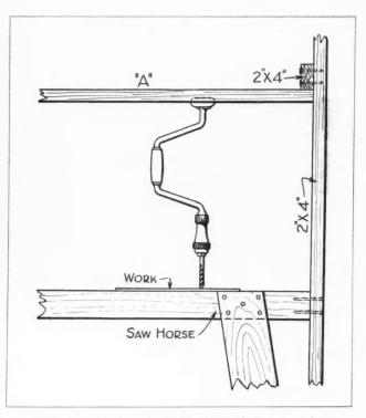
Extra leverage given by "A" in boring holes in metal.
