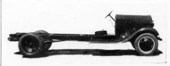
New truck chassis has flat-faced cowl at no extra cost.
