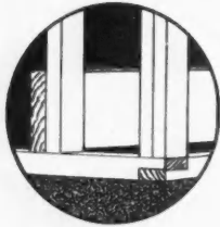
1. Plates and corner posts.
