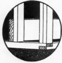
1. Plates and corner posts.
