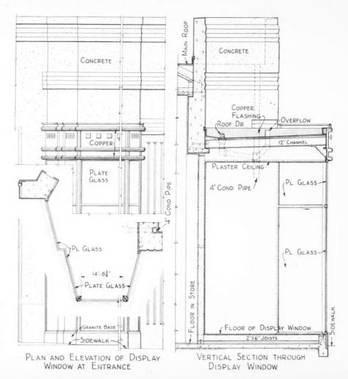
AT RIGHT: Plan, elevation and section drawings of the display window at the entrance of the Switzer Store showing modern design treatment of these projecting units. The copper fronts are finished in verde antique to contrast with the white concrete building walls.
