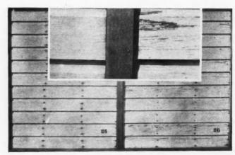
Figure 3, Sections of Southern Yellow Pine Siding after 4 years' Exposure; Aluminum-primed lumber on left, white-primed lumber on right; Close-up insert shows typical type of paint scaling.
