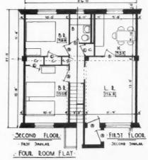
PLAN NUMBER HD-42; 3and 4-room flats; type of plan: ribbon unit with balconies; characteristics: a flat house of interlocking type, off-center column construction, bathrooms same throughout, used as a ribbon, with basements optional, efficient plumbing layout with stacks grouped.
