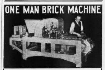
Offers one man in each locality an outstanding manufacturing opportunity. Makes a superior trademarked building unit that brings permanent fireproof construction down to the cost of frame. Uses local materials and labor, and produces 32 brick per minute. Same machine also makes single, double and triple units.
