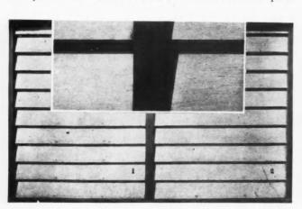
Figure 2, Sections of Edge-grain Red Cedar after 4 years' Exposure; Aluminum-primed lumber on left, white-primed lumber on right; Close-up insert shows condition of the two surfaces.
