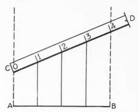
Let AB be any dimension to be divided into a number of parts. By using a scale, CD, of equal parts, the same in number as the desired number of sub-divisions, but a little larger, and holding this scale obliquely between the extreme limits of space, AB, the line is easily divided into any number of sub-divisions by drawing perpendiculars to AB through points 1, 2, 3, etc.
