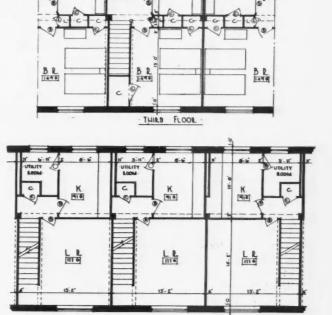
PLAN NUMBER HD-44; 3- and 4-room three-story combination houses; type of plan: ribbon unit; characteristics: a combination flat and row house plan type with 2-story row house superimposed over a 1-story flat, off-center column construction, bathrooms same throughout, used as a ribbon, with basements optional, efficient plumbing layout with stacks grouped, units can be reversed.
