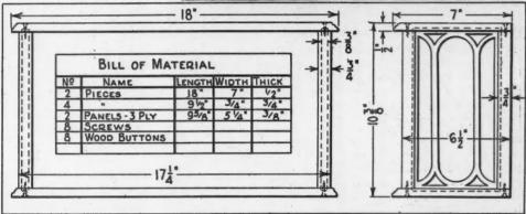
RIGHT, ABOVE: The illustration and drawings show a hanging bookshelf, a popular and useful small piece. Below: Working drawings for a day bed; the width can be increased to make it a larger size. A wooden upholstery frame will serve instead of a spring if used for a couch. Designs from E. F. Worst.
