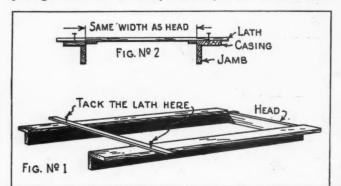
METHOD for holding jamb square while installing.
