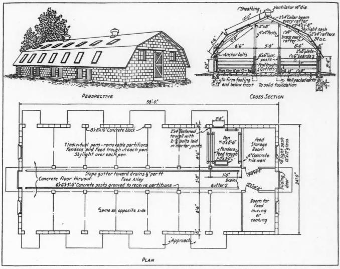
ROOF-LIGHTED hog house of cement block construction, drawing No. C-2169, from the Portland Cement Assn., Chicago, and presented in the helpful book, free on request, "Plans for Concrete Farm Buildings."
