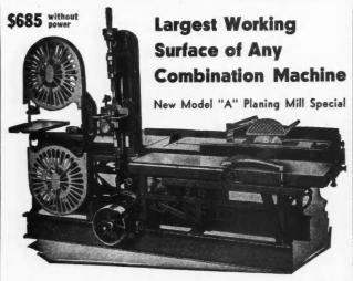
Under the FHA Plan you have three years to pay for this necessary equipment. Eight machines in one—each independently operated. All bearings high-grade ball bearings. Write for complete details of the FHA Plan.
