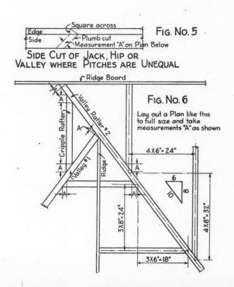
To get the position of the valleys where the pitches are unequal proceed as follows: The pitches of the main roof are 12 inch rise to 12 inch run, and of the south gable 16 inch rise to 12 inch run. The south gable ridge will be 6 times 16 inches, or 8 feet in height, the main roof having a rise of 12 to 12 run. Then the ridge will meet the main roof back 8 feet from the main
