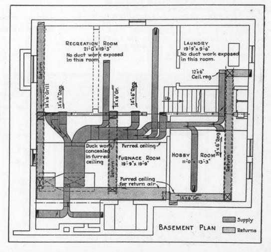
LAYOUT of basement with warm air supply and return ducts for Gar Wood air conditioning plant. Rooms are left unobstructed.
