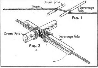
TWO poles and a piece of rope used to give powerful pull.
