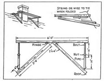
DRAWINGS of adjustable roof jacks.
