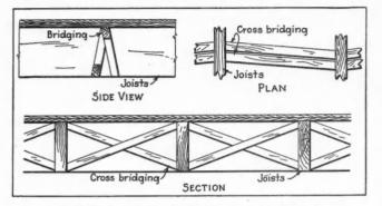
DRAWINGS of cross-bridging joists to stiffen old floors.
