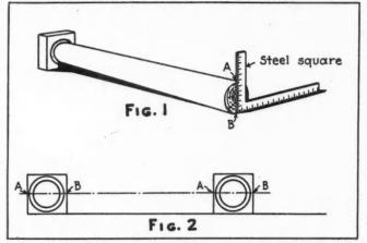
SETTING columns so that cap and base are parallel.
