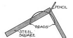
DIAGRAM I: How to draw a semicircle with the steel square.
