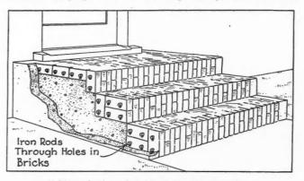
IRON rods through bricks hold steps together.
