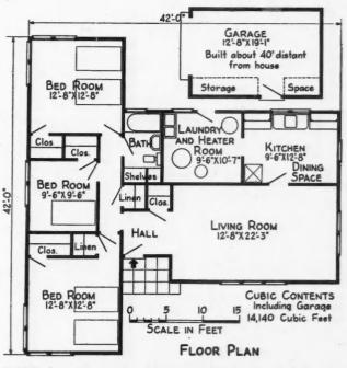
FLOOR plan of House No. 2 with detached garage; cubic contents, including garage, 14,140 cubic feet; contract price \$4,625; unit cost 33 cents per cubic foot.
