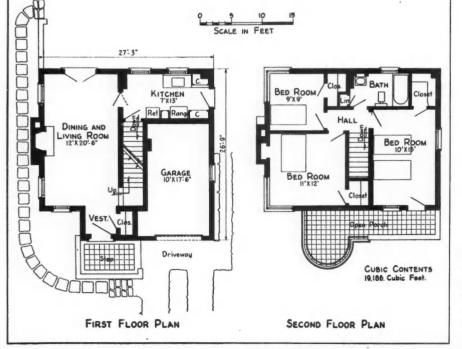
FLOOR plan of House No. 3 as illustrated on opposite page in wall section and perspective sketch. Snapshot of basement excavating activity (under canvas tent) on page 75. Cubic contents 19,186 cubic feet; contract price \$4,997; unit cost 26 cents per cubic foot.
