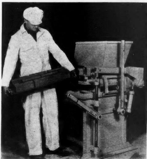
ABOVE: Machine developed for casting six-brick unit, corner unit, single brick and half brick at one operation.
