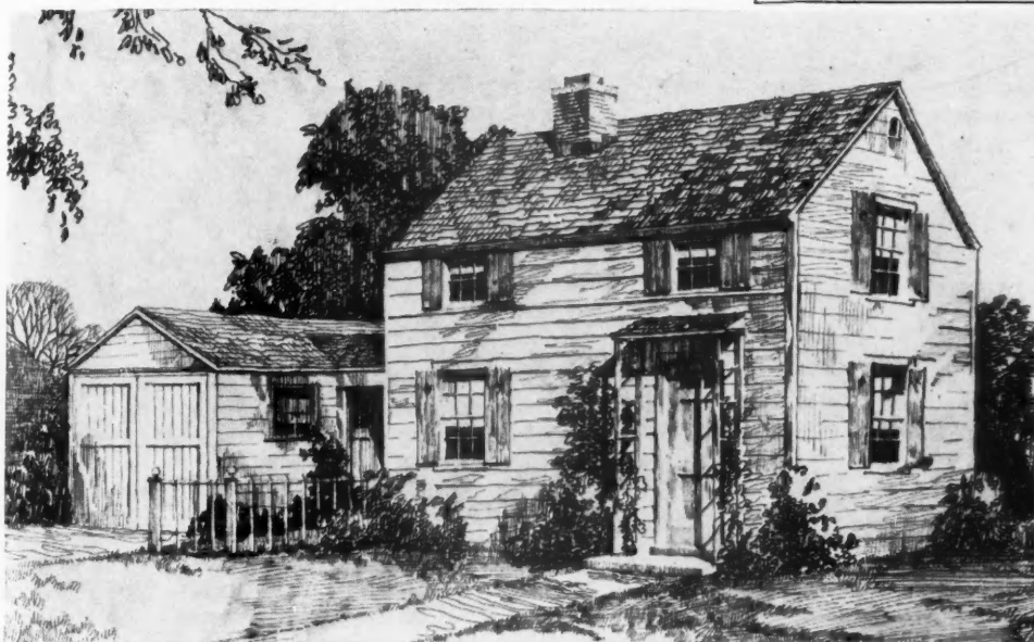
EXAMPLE D groups the rooms which are similar to house C so that the principal outlook is to the rear. Hall space is reduced to a minimum; alternate first floor plan provides a dining alcove if a basement is added. Cost Range, $1750-$2100. Cost Key is .907-81-394-18-14-5.
