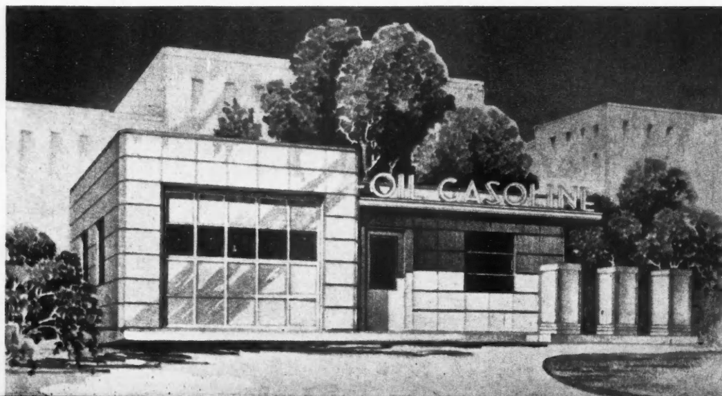
LEFT: Design for modern station using Rostone, a processed composition stone which is molded in slabs of varying thicknesses from one to two and one-half inches and cut to specified dimensions.
