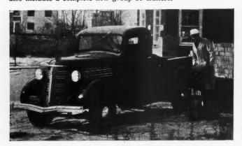
THIS pickup model in 1937 line of GMC trucks has 1/2-ton capacity.
