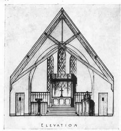
ABOVE: Elevation of chancel as seen from church nave; roof trusses are of wood. The detailed plan of the chancel is indicated at the right and is inverted in relation to the position it occupies in the street end of the church as indicated in the main floor plan below at the right. Facilities as arranged in the plans fill the requirements of present church programs of religious education and other activities.
