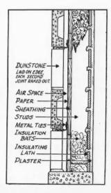
LEFT: Wall section showing concrete block veneer. Below: Load-bearing corner window post section.
