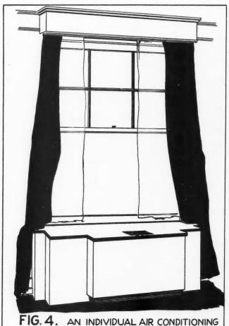
FIG. 4. AN INDIVIDUAL AIR CONDITIONING AS USED IN A HOTEL ROOM. THIS IS SERVED FROM A CENTRAL SYSTEM
