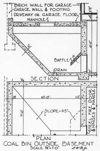
CROSS-SECTION of concrete bin and reinforced shovel-box baffle, with metal door, constructed outside of foundation walls.
