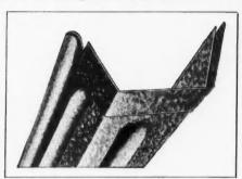
HANGING eaves trough for box gutter effect.
