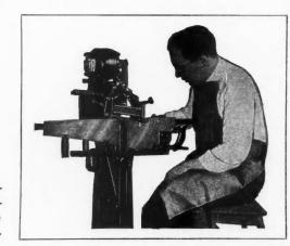
FOLEY automatic saw filing machine in operation.
