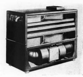
AIR conditioning dehumidifier of silica gel type.
