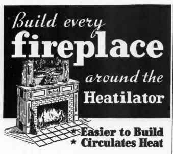
THE Heatilator is a steel heating chamber hidden in the fireplace—a correctly designed form for the masonry that insures SMOKELESS operation. Complete from floor to flue, including well-proportioned firebox, smoke dome, damper and down-draft shelf, it greatly simplifies construction—saves materials and labor.
