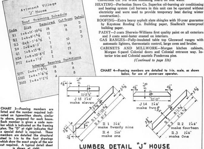
listed and the number required indi-cated on typewritten sheets, similar to above, prepared for each house. Each member is given a code number which is indicated on the framing plan. The "D" at right indicates that a special detail is required. These members are detailed like structural steel in I-in to the foot drawings which show the exact angle of the saw cut required. A typical detail sheet is shown at right.
