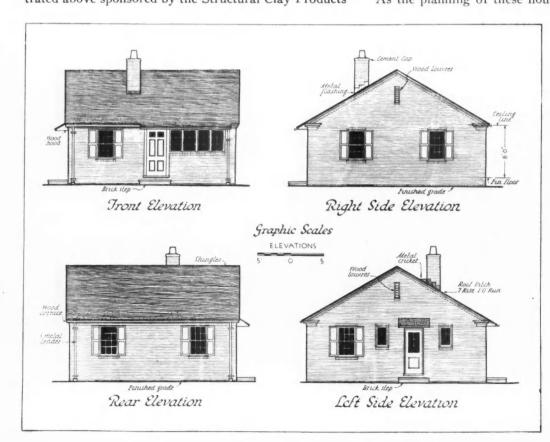
DETAIL drawings of the low-cost FHA "B" house showing construction in brick as recommended by the Structural Clay Products Institute.
