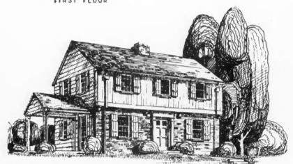
Exterior Walls: Wood siding exposed 8½ to the weather on side and rear walls, building paper, shiplap on 2 x 4 studs 16° o.c., plaster on wood lath; 4° brick veneer on lower half front wall; vertical siding on upper half front wall.
