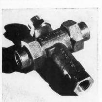
fresh water safety seal in any drain trap, regardless of how infrequently the drain is used. The Phillips automatic valve is set into the cold water supply line running to a frequently used fixture. It "bleeds" enough fresh water to maintain the required fresh water seal. Back siphonage is prevented.
