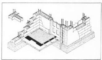
MORTARLESS block system of reinforced construction.
