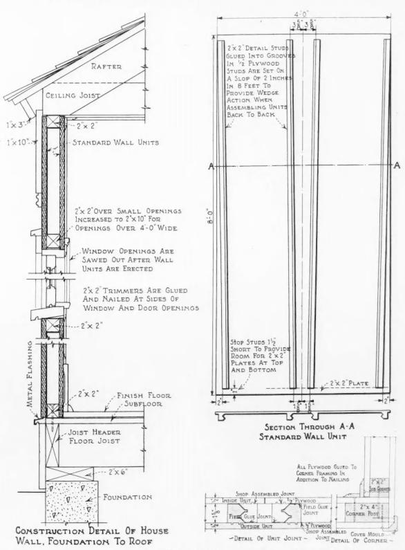
DETAILS of Horn Wall Units and how they are used in one-story wall construction.
