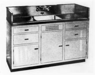
THE 1926-29 ELKAY SINK in white metal or monel metal had a 25-gauge top built over a solid wood frame. All joints were soldered and the seams were visible. Although it offered resistance to stain and acid, denting, scratching and tarnishing, it was only half as thick as the 18-gauge stainless surface used in 1937 sinks. Now the reinforcing is 14-gauge steel backing, making a total metal thickness of over 1/8 inch. Basins are butt welded flush
