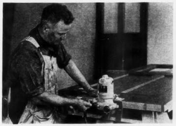
PLANING and fitting doors, sash and transoms are done quickly and inexpensively with this electric door plane. It will cut 1/8 inch off a 7-foot hardwood door in less than a minute.
