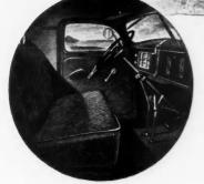
The ALL-STEEL CAB is a feature in every new International. The one-piece top, the sides, the back and cowl panels are welded into the complete cab frame. Rubbermountings wherever cushioning is needed. This is the roomy, well-appointed de luxe cab.
