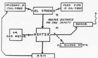
THIS detailed diagram shows the various factors that should be considered in planning arrangement of heating equipment. By preparing diagrams of this kind, mistakes will be avoided and more satisfactory and practical layouts will be made.
