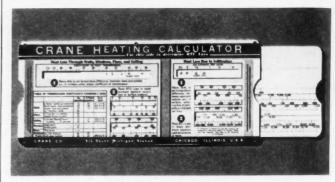
SLIDING scale saves time, gives accuracy in figuring heating.
