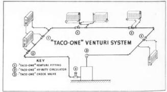
NEW ONE PIPE hot water heating system.
