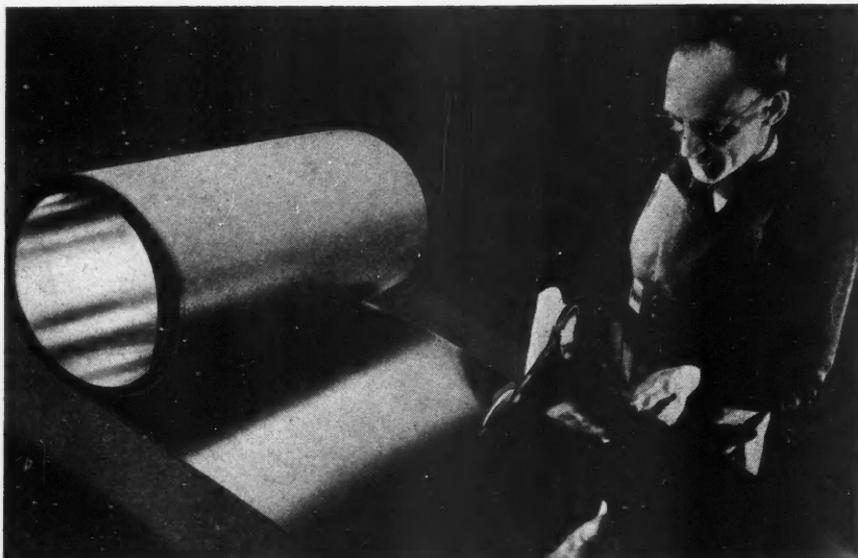
NEW STAINLESS STEEL PRODUCT is easily handled and cut with ordinary heavy shears.
