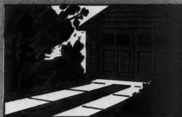
(Below) RIBBON CONCRETE DRIVEWAY
