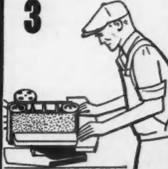
3 AS A SPINDLE SANDER—Concave surfaces are sanded quickly and efficiently at front pulley of sander when used with bench stand.
