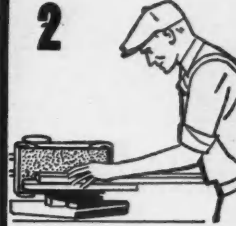
2 AS AN EDGE SANDER—Used with the bench stand. It becomes an ideal edge sander for pieces too small for a portable tool
