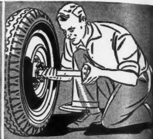
Full-floating rear axle relieves the axle shafts of supporting the weight of chassis and body.
