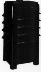
The new unit is of the Heat-Director type, supplying both radiating and circulating heat. Adjustable shutters on three sides make it possible to direct heat downward to warm the floor. The company's Heat-Directors are finished in porcelain enamel, and the radiating heaters in either porcelain enamel or polished steel. They are adapted for operation with either No. 1 or No. 2 fuel oil and can also be operated successfully with either kerosene or distillate.
