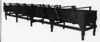
This machine uses the new modern principle of VIBRATION which assures Super-Dense concrete Units. 240 ft. of Joists can be produced in one operation, at low labor cost.
