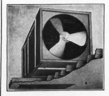
PHANTOM-VIEW with joist cut away to show fan unit and suction box connected with ceiling grille.
