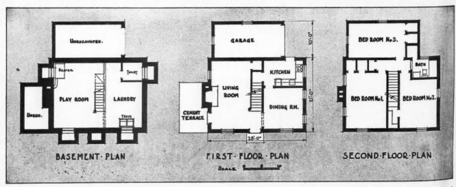
FLOOR PLANS of the Aronimink Estates model home shown at extreme right, above. Rooms are spacious, well arranged, with attached garage at rear; the third bedroom is located above garage giving compact second floor layout.
