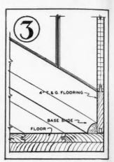
inch flooring used as a flush base (see Fig. 3). This feature also provides concealed nailing, hiding the nail heads in the depth and shadow of the joints where they get a good grip on the material and a firm hold on the studs.
