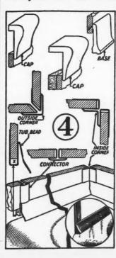
LEFT: Factory-finished board in plain, tile or patterned surfaces for use in kitchen or bath can have joints either filled or covered with metal moulding. This detail shows a method of using mouldings to give a good, tight job around a bathtub. (Monewall detail.)
