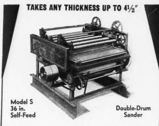
Sanding Drums 19 in. diameter. Feed Rolls cold rolled steel—4 lower and 4 upper rolls, all power-driven. Bed Plate takes material as thin as  $\frac{1}{12}$  in. and as short as  $7\frac{1}{12}$  in. with perfect alignment and even pressure. Sand Disc 18 in. dia.
