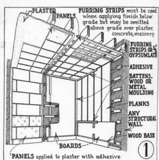
RECOMMENDED application procedure for boards, planks, panels and tile on different types of wall. (Armstrong detail.)
