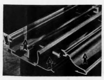
OUTSIDE INSTALLATION is a feature of Pittco Metal vitally important to speed and ease of application, and to glass replacement in the future. As shown, the inner member (1) is set; the setting block is pressed into its groove and the glass lifted into place (2); then the glass holding member is installed (3); and finally the face member (4) snaps on to finish the assembly.
