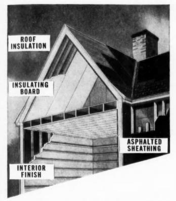
which are themselves waterproofed in manufacturing, asphalting provides an additional weather and moisture proofing which seals both the sides and edges of the board. A bright aluminum powder coats one side, providing further protection. Asphalted C-S-I Sheathing adds to the salability of the houses you build by providing a moisture and vapor resisting barrier plus added structural strength and insulation.
