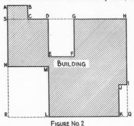
the distance EF equals the distance CD, the work is proved to be correct. If either of these fails there is an error and work must be repeated until it checks.
