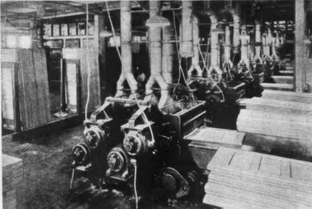
Since the introduction of dowel machinery about 40 years ago, stock doors have been made almost entirely with dowel construction. Since doweling lends itself to large-scale production by its very nature and permits of greater material economies, it is now virtually standard construction, especially in the large factories. The advance in the technique of doweling, particularly the development
