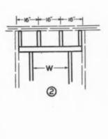
BASIS for determining lengths of standard framing members is indicated in this sketch, used in connection with formula described in accompanying article. Lengths of stud and header are guiding factors.
