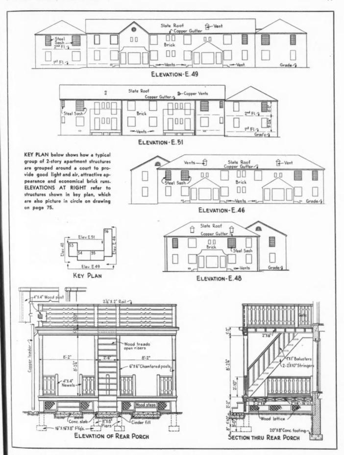
SIMPLE ARCHITECTURAL LINES, long uninterrupted well areas shown in elevations above reduce brick laying costs on Lindcrest houses.
