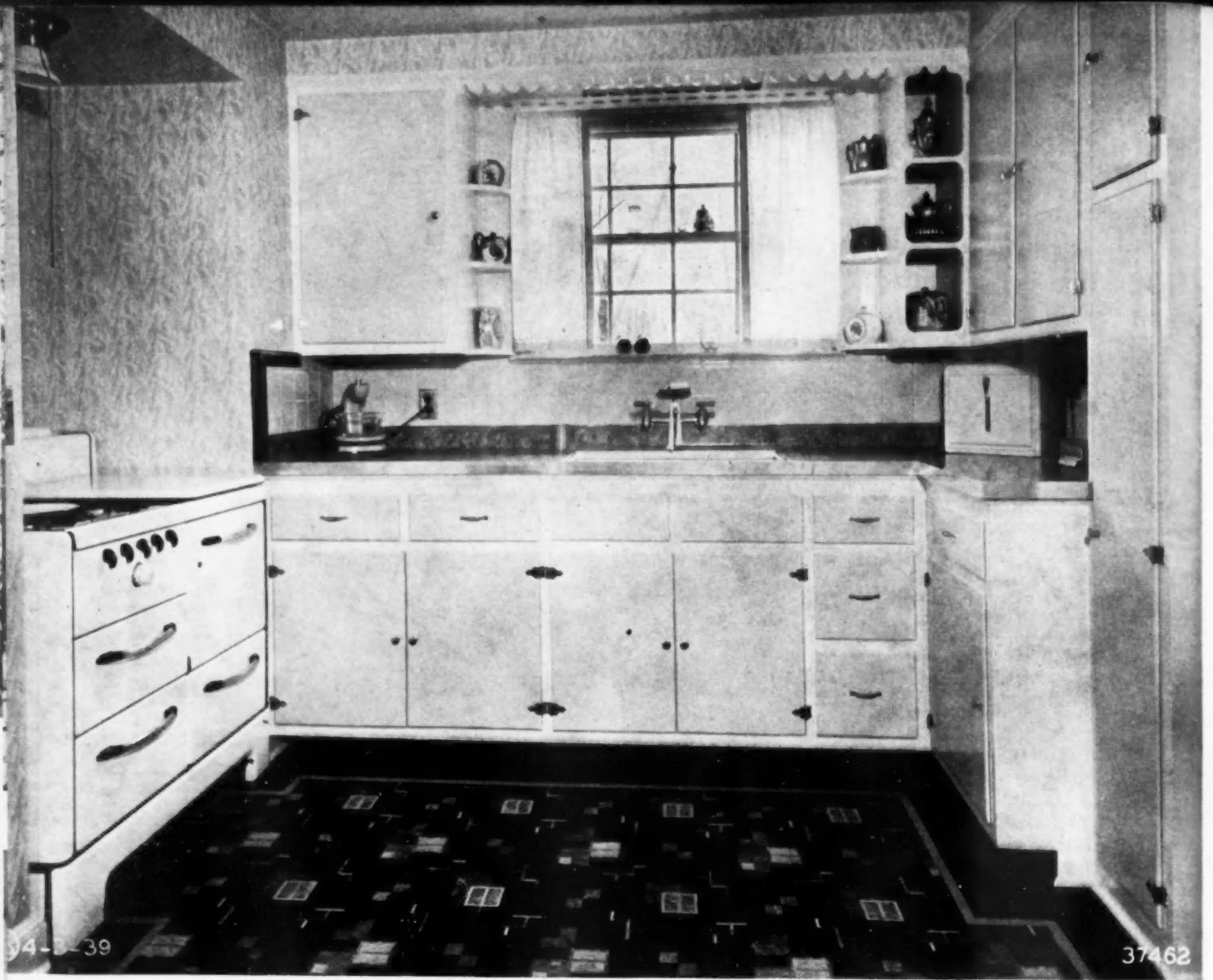
KITCHEN is laid out in efficient U-shape, with gas range recessed in well-lighted alcove.
