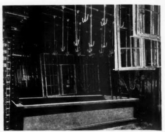
STEEL windows ("Fenestra") on moving hooks are dipped in a series of preservative baths in the Bonderizing treatment.
