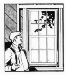
SET UNIT in wall. Units are set in wall simply by nailing wide blind stop to studs. This type of overlapping joining insures a weathertight wall joint.
