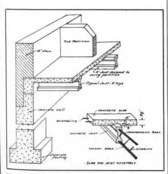
ECONOMIC, firesafe construction, as used in Tasker Street project of U. S. Housing Authority in Philadelphia. The machine-rolled concrete joists, on 30-in. centers, are bonded to the 21/2-in. floor slab. No plaster is applied on under side of second floor. Concrete joists were made in plant of the Formigli Corporation, Philadelphia.
