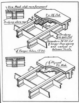
TWO methods of placing floor slab forms with Lith-I-Bar joists.
