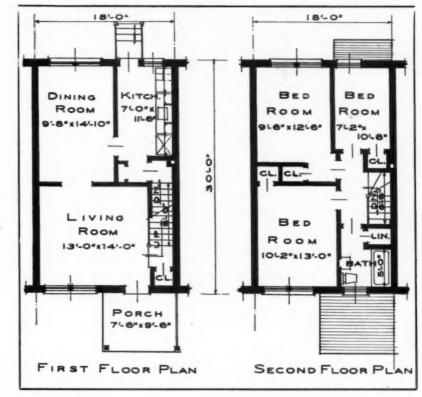
NINETY-FIVE of the above low-cost Argonne Drive row houses were sold in less than two months by Meyerhoff's Columbia Construction Co. Typical plan, 18 by 30 ft.
