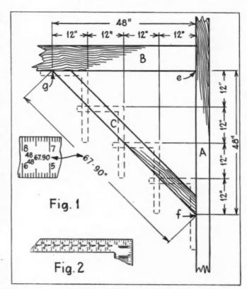
FIGURES 1 and 2 illustrate method of using the brace measure.
