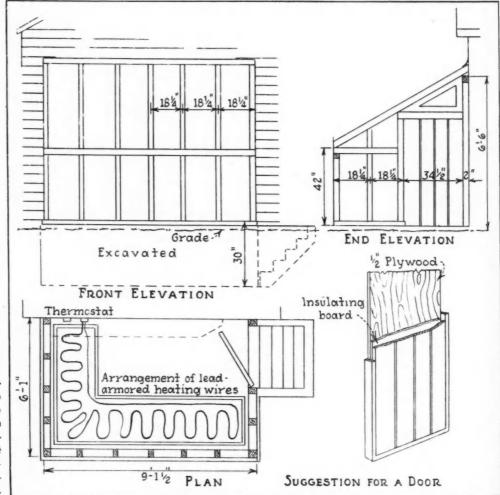
PLAN and elevations of inexpensive greenhouse built along the side of the garage or home. The framing is spaced to take 36-inch wide wire glass which allows construction economy; cuts down heat loss because of dead air space between double facing; admits ultraviolet rays; eliminates breakage. he
