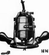
Mortises for butts 6 times faster than is possible by hand. Direct drive ½ H. P. motor runs at 18,000 R. P. M., cuts quickly, smoothly, accurately — leaves flat, even surface assuring perfect fit every time. High speed of cutters prevents tearing out wood between mortise and door edge. Used for all butt and lock face mortising.
