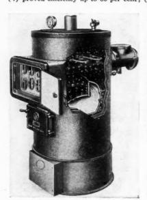
transfer a maximum amount of heat to water -stack temperature as much as 1000 degrees lower than many; (6) water coil for domestic hot water ready installed; (7) doors insulated with refractory lining or baffle liner, and door castings with gas-tight ground joints, or grooves sealed with asbestos rope gasket; (8) all flues easily accessible from the front for quick, easy cleaning.
