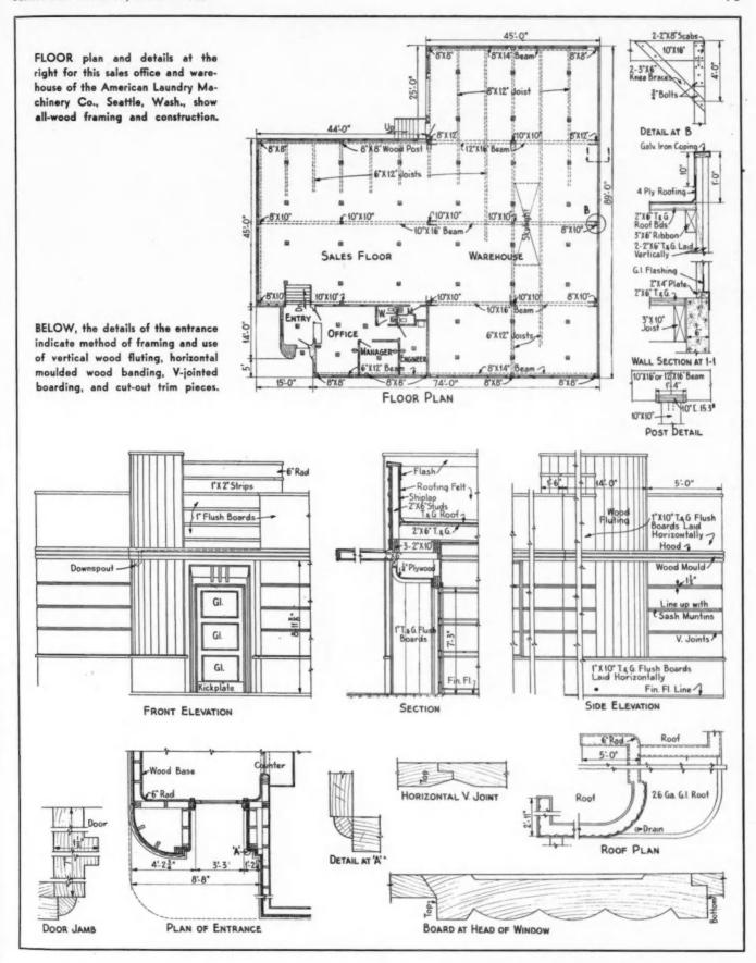
covered with metal lath and plaster. Salesroom walls are finished with ½ in. 3-ply plywood, and walls in the office are finished with scored plaster and oil painted in flat tones of cream and gray. Except in the office, where Tile-Tex asphalt tile flooring is used, all floors are finished with 2 x 6 T&G fir, sanded.
