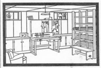
Waste space in the cellar can be used to make this practical workshop. Tempered Presdwood is ideal for walls, ceilings, shelves and cabinets because it is highly moisture-resisting. Even though the cellar may be damp, Tempered Presdwood will not warp, chip, split or crack when it's properly applied. Walls and ceiling are grooved with U scoring, and painted white.
