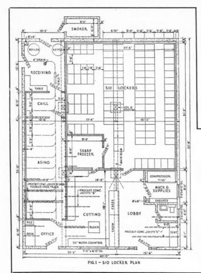
FIGS. I and 2 at left and below show a typical floor plan arrangement for a 510-locker plant and a section indicating construction and method of insulation.
