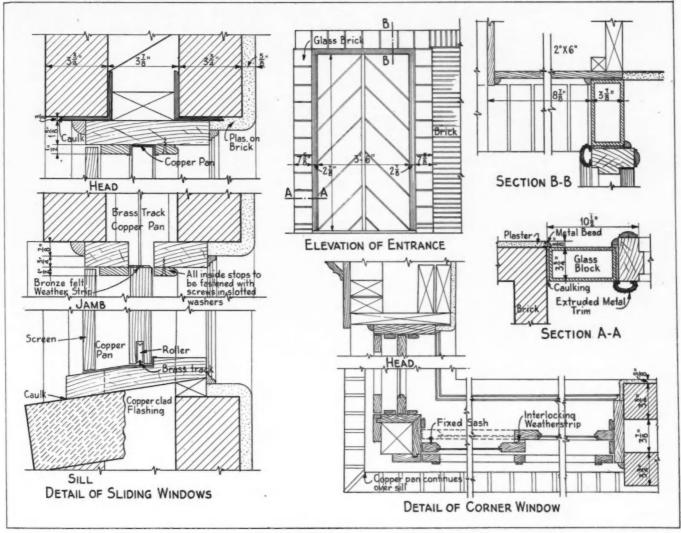
THE above details show hollow wall construction carefully flashed around openings; sliding windows run on special track into space between inner and outer walls. The front entrance has a modern treatment with glass block flanking the jams and across the head.
