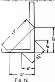
the piece of stuff) until the 8½ inch mark on the outside edge of the blade is on the line previously drawn along the outside edge of the tongue (line C-D in Fig. 11). The square will then have been advanced 81/2 inches further in the direction of the run of the hip rafter and a total distance in this direction corresponding to the 12 foot six inch. run of the common rafter. With the square in this (Continued to page 98)
