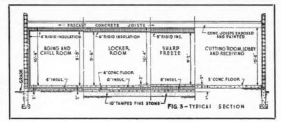
room, floors, walls and ceilings, 4 in. of insulation; in the locker room 6 in. of insulation in floor, walls and ceilings; in the sharp freezer, 8 in. in the floor and ceiling, 8 in. in walls facing a room which is held at normal room temperatures and 4 in. in walls facing a refrigerated room such as the locker room. Sharp freezer walls facing the chill room or aging room are usually built with 5 in. of insulation.
