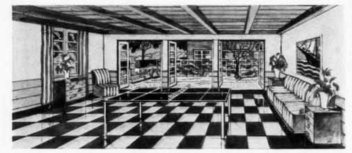
THE perspective drawing indicates the view which will be seen from these Blue Island houses as looking from the recreation room through the three pairs of French doors out into the sunken garden courts. Note the beamed ceiling effect by use of 4 by 8's and beaded 2 x 6 subflooring.
