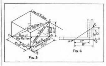
from an Architect's drawings, he can measure off from the sectional or elevation drawings to scale the *span* of the roof and the *rise* of the roof. The *run* of the roof will be  $\frac{1}{2}$  of the span and if the *rise* of the roof *in inches* be divided by the *run* of the roof *in feet*, the result will be the *rise-per-foot-of-run* for the roof.
