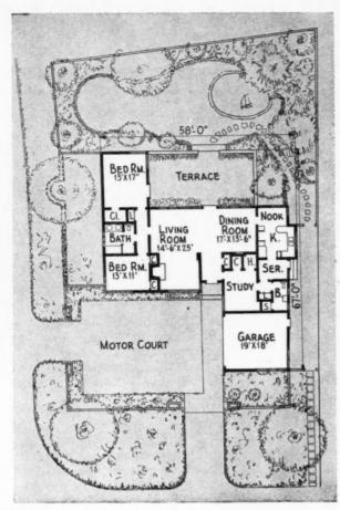
PLOT and floor plan above shows well considered placement and arrangement for light, air and view in Hollywood home designed by Sumner Spaulding, architect.
