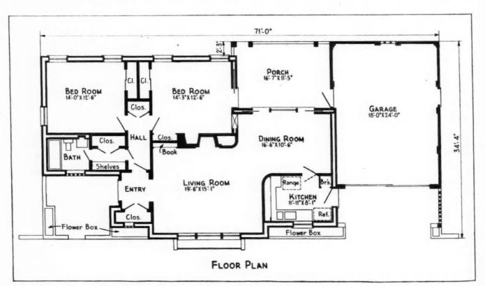
PLAN indicates the use of hollow brick walls with four-inch air space; they are built up on a reinforced concrete floor slab. The large closed-in porch has access from three sides. Note that three of the doors slide into the hollow walls.
