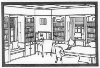
Ace high is this card room-library. The flexibility of Masonite Tempered Presdwood permits several unique features. For walls and ceilings the board can be left natural, or painted or varnished. Radio loud-speaker is installed behind a Tempered Presdwood panel over built-in desk. Ample bookshelf space is provided by using Tempered Presdwood for cabinetwork.
