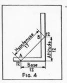
hip rafter. But the run of the hip rafter is  $\frac{17}{12}$  times the run of the common rafter and therefore it can be said that the rise per 17 inch run of the hip rafter is always the same as the rise-perfoot-run of the common rafters for roofs of equal pitch. If the rise of the common rafter perfoot-of-run is eight inches, then the rise of the hip rafter for each
