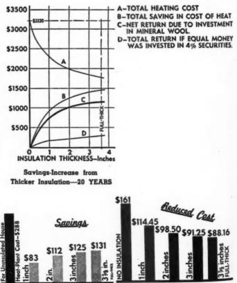
Savings in Heating Plant First Cost when house is insulated.
