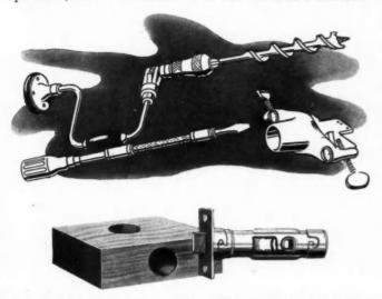
Brace and bit, screw driver and bit guide are the only tools needed for installing a tubular door lock or latch.
