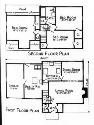
WHILE the exterior styling of the house below gives it an entirely different appearance from the one above, the floor plan is quite similar; the three bedrooms are larger, however, one replacing deck over wing.
