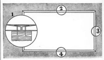
INSERT in above illustration shows how taped joints can be made on all four sides of new bevel edge wallboard.
