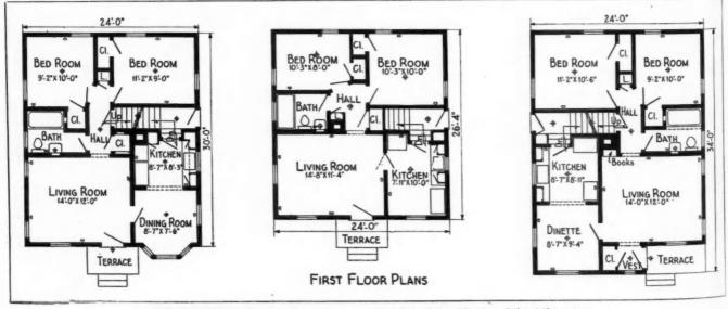
THREE TYPICAL Garling floor plans, ranging from 24' x 26' 4" to 24' x 34' in size.
