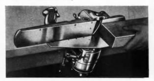
Other features: Spiral Cutter makes smooth, waveless cuts with or across the grain without splintering the edges. Quickly Adjusted for paper thin or heavy cuts up to  $\frac{3}{16}$  of an inch. Sharpens its own cutter.
