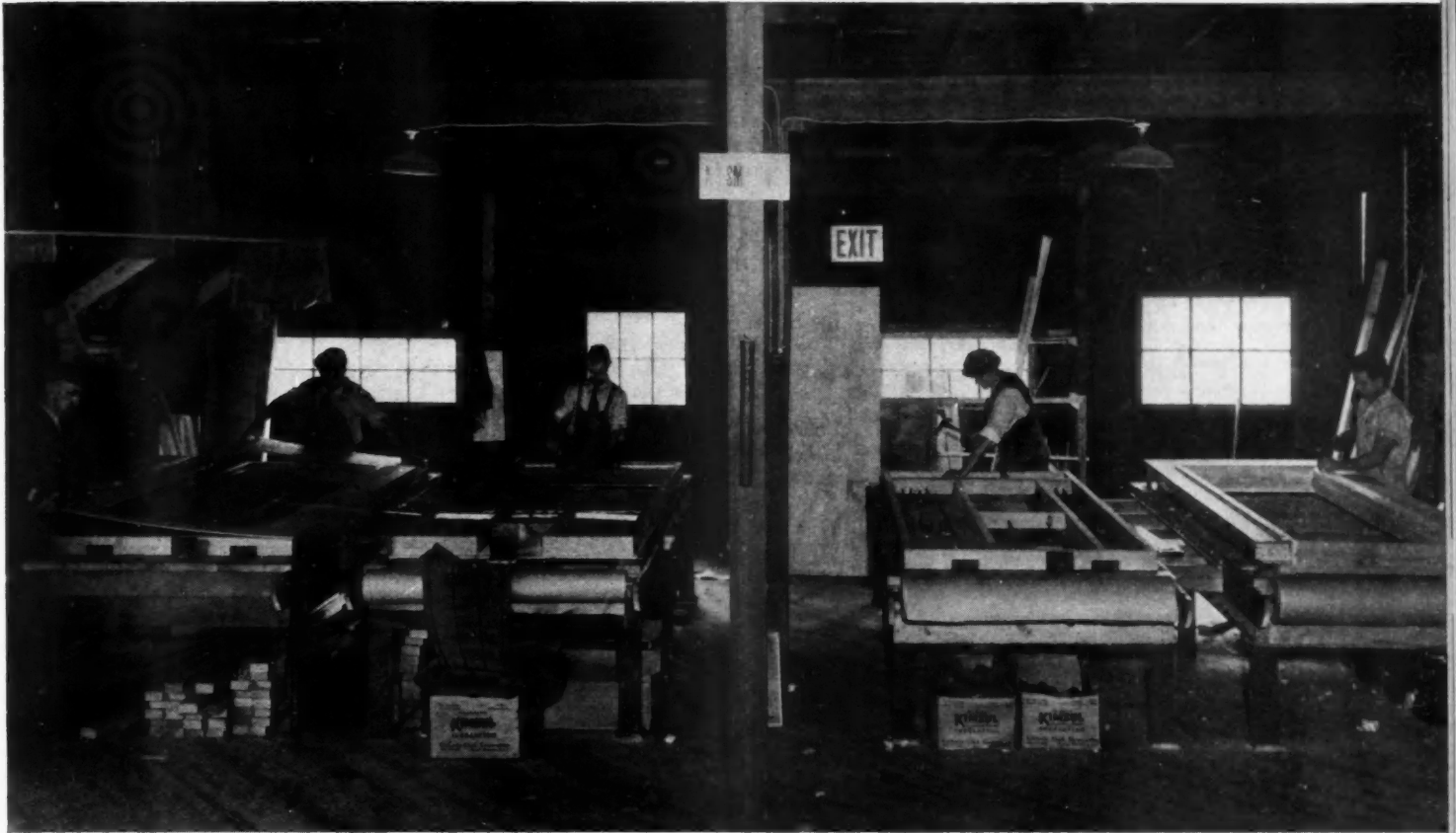
WHYTE'S WORKSHOP where wall panels are built under controlled conditions. Angle irons on tables hold studding in place as plywood is "stretched" and nailed. Rolls of building paper and blanket-type insulation are convenient; at far right, putting on interior door trim.
