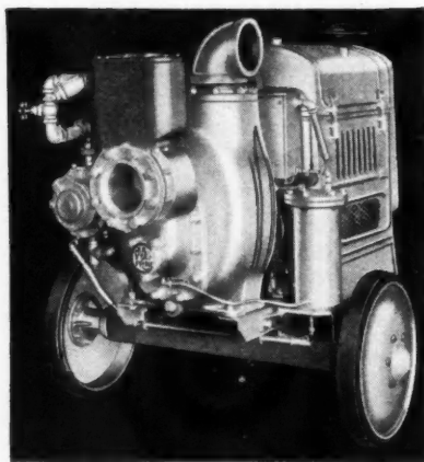
CMC Well Point Pre-Drainage Pump.
