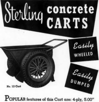
x 21" Pneumatic Tires; Roller Bearing Wheels; 12 Gauge Welded Tray with Heavy, Continuous Tray Rod; 9 Cubic Feet Level Capacity; Heavy, Flanged Legs, Welded to Tray; Alloy Steel Underslung Axle.
