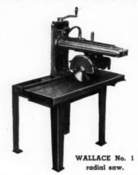
ripping, shaping, rabbetting, tenoning, dadoing, grooving and many other milling operations. It is designed to permit cut off and angle work on both the "push" and "pull" strokes of the motor alternately. New geared motors of one or two h.p. have a spindle speed of 4900 r.p.m.,—adequate for fine shaping and routing work,—and with blade capacities up to 11" in diameter, cutting up to 4 inch material.
