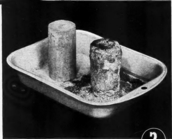
was put into the tray and the cylinders were alternately frozen and thawed 15 times. Note in photo 2 that Brixment mortar remains intact, whereas the other mortar has crumbled badly. This simple test can be made in any ice-manufacturing plant.
