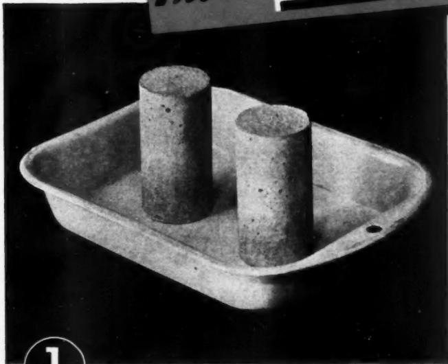
Above: A cylinder of Brixment mortar (left) and a cylinder of mortar made with 50-50 cement and lime mortar (right). Both specimens were made at the same time, and subjected to exactly the same treatment. After curing for 30 days, \frac{1}{4} " of water
