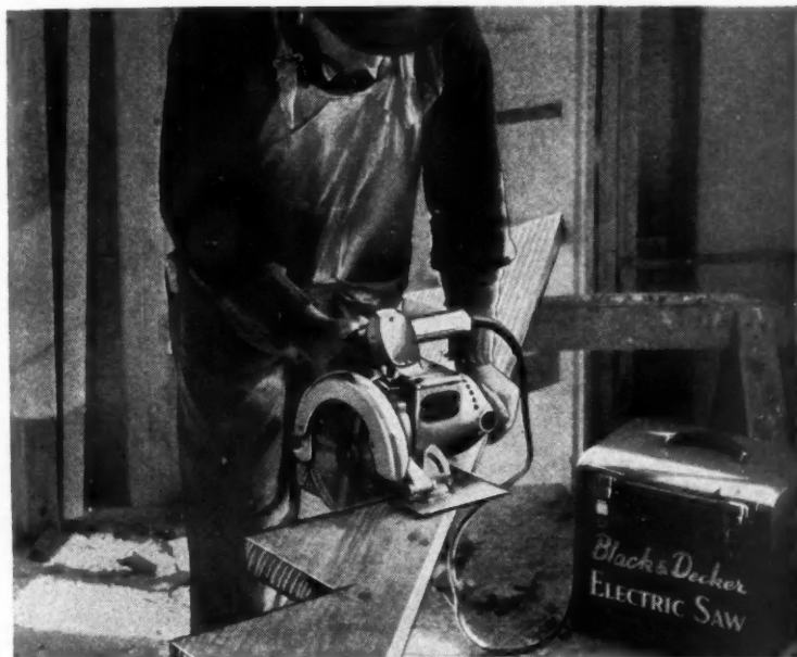
CUTTING STAIR STRINGERS in a fraction of the usual time with Black & Decker No. 85 Electric Quick Saw—famous builder's saw with easy one-hand operation.
