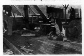
AT FACTORY, floor sections are built two at a time, cut apart by power saw. Units are insulated with  $\frac{1}{2}$ " blanket, have factory-finished oak floor surface.
