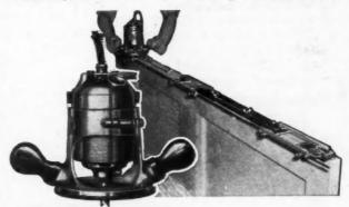
MORTISE FOR BUTTS in door and jamb with Carter Hinge Butt Router. Accurate depth adjustment up to 1½". ¾ H.P. motor turns cutting bit at 18,000 R.P.M. Used with Hinge Butt Templet No. T4 for butt mortises, with Lock Face Templet No. T1 for lock face plates.
