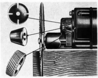
The patented Shock Absorber of the Walker-Turner Geared Motor protects its gears against breakage during momentary overloads. The spring-tempered steel washer, under tension, relieves strains on gears and resets itself.
