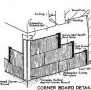
NEW J-M asbestos shingles and how laid without face nailing.
