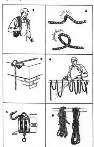
1. Carry rope—don't drag it; 2, keep free from kinks; 3, pad sharp corners; 4, clean off mud; 5, use blocks of proper size; 6, coll and hang for storage.
