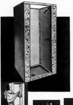
This non-metallic shower stall conforms with item P-19-A War Department specification PE-623 and uses a minimum of critical materials. The walls are of fibreboard, baked-on enamel finish, and metal parts are galvanized steel. The receptor is precast concrete with integral drain. Size 32 by 32 by 75 inches.
