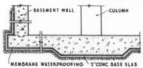
Basement slab designed for hydrostatic pressure.
