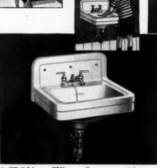
• CE-764 new "Victory Cantonment" lavatory. Made of easily cleaned vitreous china with cast iron trim, heavily galvanized. Mounts directly on the wall with screws—no hangers needed. Uses a minimum of critical materials.
