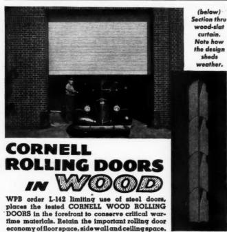
Also ask about Cornell Wood Vertical-lift doors, Canopy and Bi-fold doors. Cornell Wood Rolling Doors consist of interlocking wood slats, strung on metal bands placed 2' to 3' apart, and operating plywood guides, with light formed-plywood hood covering the coil. Weather-protected. Can be motor operated.
