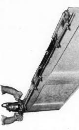
D. Rout recesses for butts. Door on edge, T3 templet hinged to bench. Use Carter Butt Router.
