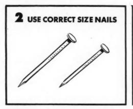
WHY? Nails must conform to the thickness of 18-inch shingles, use 1½-inch (three-penny) nails. For 24-inch shingles, use 1½-inch (four-penny) nails. Be sure that nails are rust-resistant. When shingles are nailed as directed in No. 3, the overlapping of the succeeding courses completely covers the nails and protects them from the elements.
