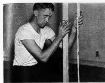
Placing 30" thermocouple in position
