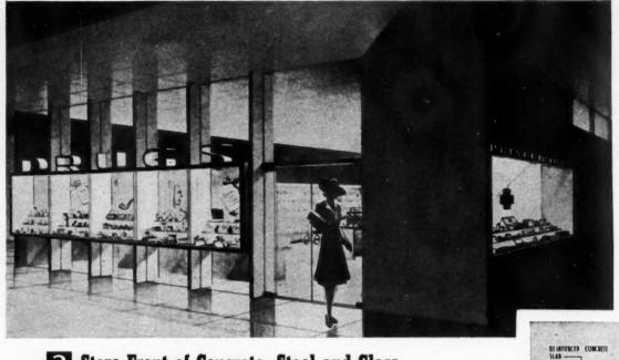
THIS perspective shows the corner of the drug store in the five-shop plan below. It has a protecting marquee in the form of projecting reinforced concrete roof slab, that shelters the varied lcb. bies. (See side elevation.) Window display units are set between the vertical precast stone slabs and are fluorescent lighted as detailed below. The balance of the store front is glass, including the entrance doors. Designed by M. Righton Swicegood, New York City.
