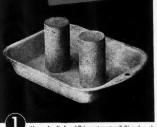
Above: A cylinder of Brixment mortar (left) and a cylinder of mortar made with 50-50 cement and lime mortar (right). Both specimens were made at the same time, and subjected to exactly the same treatment. After curing for 30 days, 1/4" of water
