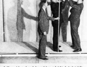
A 50-pound bag of sand dropped from a height of six feet fails to harm a Strong-Bilt Panel supported on centers 28 inches apart. Strong-Bilt Panels withstand impact blows up to 6 times that of boards with a mineral core.
