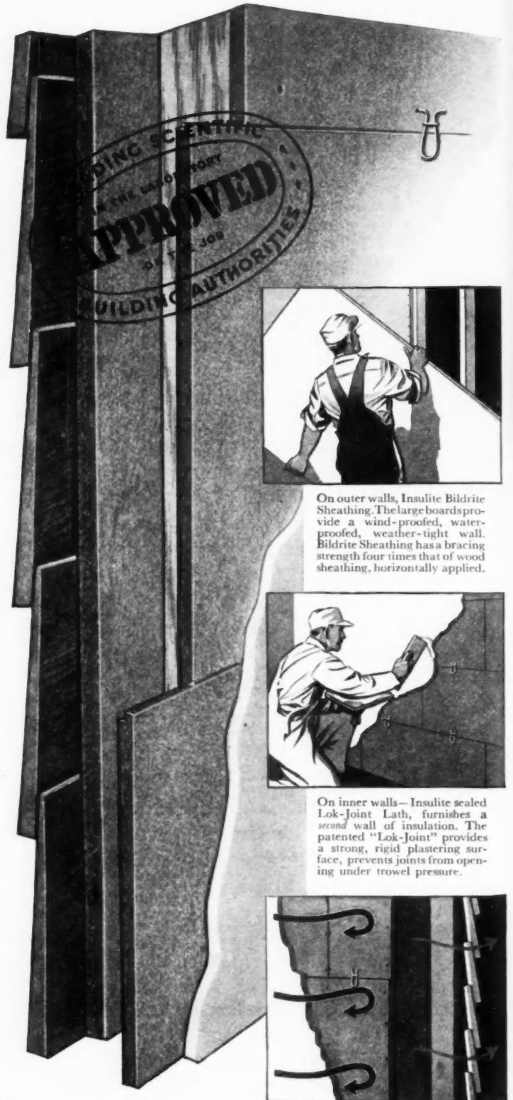
How moisture condensation is eliminated in the Insulite Approved Wall of Protection: Sealed Lok-Joint Lath, with asphalt barrier against the studs effectively retards vapor travel. Bildrite Sheathing, being permeable to vapor, permits what little vapor escapes to pass naturally towards the outside.
