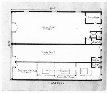
SHAPES and sizes of floor plans will vary according to types of stores.
