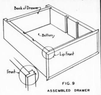
wide as the back piece is long. To assemble the drawer, glue the back into the dadoes in the sides. Keep the top edge of the back flush with the top edges of the sides. Drive 1½ in. brads through the sides part way into the back. See Fig. 9. Glue and nail the sides to the front. Keep the top edges of the sides flush with the top rabbet of the drawer front. Slide the bottom into the side grooves. Do not force it in.
