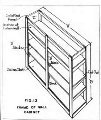
Hang the frame to the ceiling by nailing strips to the inside of the front top rail of the front frame and into the ceiling joists. The strips should be about 13% in. x 5% in. Nail the back frame to study in the back wall.
