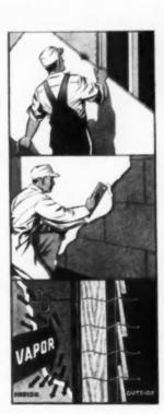
OUTSIDE THE STUDS, Insultee Bildrite Sheathing. The large boards provide a windproofed, weather-tight wall. Bildrite Sheathing has a bracing strength four times that of wood sheathing, horizontally applied.
