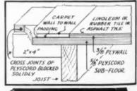
firmly, and the nails can be driven right at the edge of the panel without danger of splitting.
