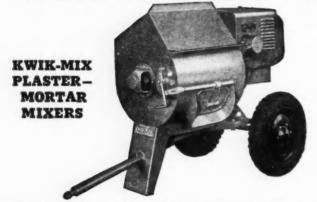
Kwik-Mix Non-Tilting 6-P Plaster or Mortar Mixer . . fast discharge, 7 seconds . . . light weight, only 850 pounds...air cooled engine...V-belt and worm drive . . . low shoveling height. Also 4 wheel 10-P tilting model.
