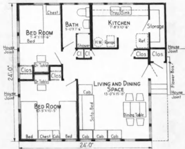
8 HERE'S FLOOR PLAN. All furniture shown was built-in at furniture factory where the sections were shipped before going to building site. Joining points show where the sections are bolted together at the site.
