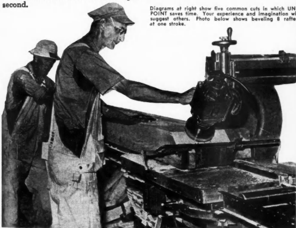
3 Instead of cutting angle (a), then angle (b), use a counter-sunk dado or rafter notch cutter and cut both angles with one stroke of saw—100% increase.
