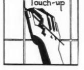
SUCCESSFUL installation of wall boards depends upon knowing just how, and this goes for all finished wallboard as well as that explained here by the installation experts of The Tylac Co. The top of wainscots must be level; if this special wallboard is sawed, do so with a fine-toothed saw and always have the finish side up when sawing. Cement the back side, nail in the scorelines, then putty, clean and touch up as shown.
