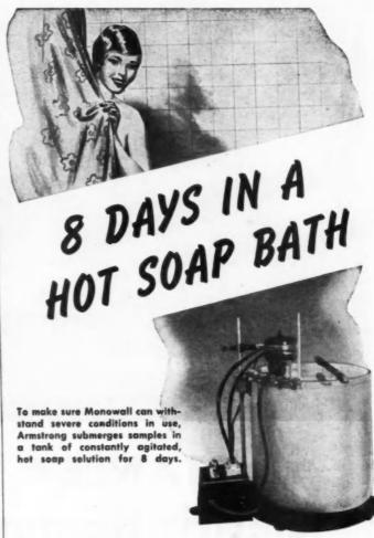
'HIS is one of the "torture" tests which Monowall must pass in the Armstrong laboratories. It establishes proof that the finish of Monowall can withstand conditions far more severe than those encountered in normal use. It proves that Monowall will give good service in bathrooms and kitchens. Splashed soapsuds and repeated washings do not affect its gleaming finish.
