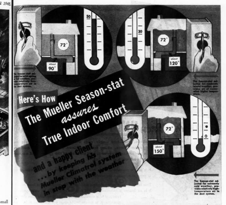
As winter weather conditions change, the amount of heat delivered by the heating plant should be changed. By controlling the air temperature in the duct system, the amount of heat can be changed. In order to provide true indoor comfort, it is essential to have continuous movement of properly heated air. The continuous delivery of air, heated to a temperature in keeping with the outdoor temperature, is attained
