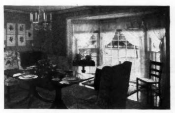
"STRETCHED" WITH A BAY—Bay windows—made up of stock Ponderosa Pine units—create an effect of greater space. Bay windows are not expensive if made of stock Ponderosa Pine units, which can be toxic treated to enhance still further the natural durability of wood.
