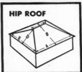
Add the eave length (A) to the ridge length (C), multiply by the distance from eave to ridge (B). This gives area of side slopes. Multiply (E) by (D), for area of end slopes. Add the two totals and divide by 100.
