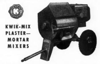
Kwik-Mix 6-P Plaster-Mortar Mixer is completely discharged in 7 seconds. Weighs only 850 pounds, easy to move. Easy to charge because of low shoveling height. Non-Tilting. Air-Cooled engine. V-Belt and worm drive. Kwik-Mix 10-P Plaster-Mortar Mixer is 4-wheel tilting type.
