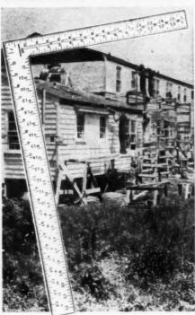
In carpentry, no tool is more indispensable than the steel square. It is more than a square and straight-edge – the markings, figures and tables of a Stanley Steel Square provide the builder with a simple calculating device for solving many problems.
