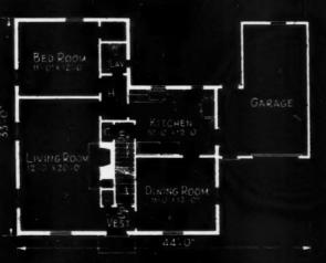
ALTERNATE floor plan directly left of this description enables builder to use plan of broad house pictured above for a narrower lot. The narrower plan is for the elevation at bottom of opposite page. Floor plans at bottom of this page are for design pictured above with two car garage. Drawings and renderings by Designer Clifford J. Foyster.
