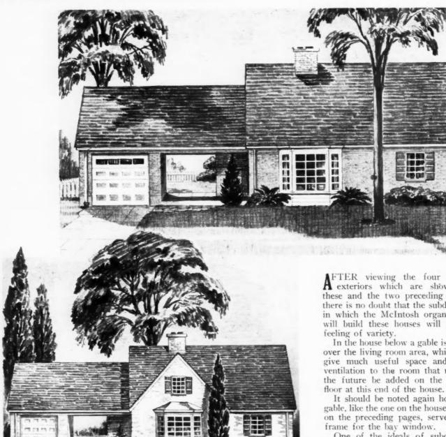
These two alternate exteriors of the basic plan with four elevations which the McIntosh organization is planning to use in one of its postwar subdivisions follow the story and a half lines of the traditional Cape Cod design. This permits use of the extra space on the second floor for additional rooms. See the detail showing the stairs going up. It is so planned that the landing will come in the middle of the second floor, allowing the building of two extra rooms with no waste hall space.
