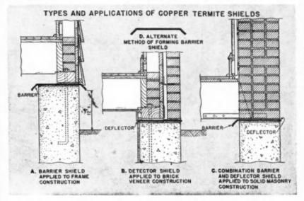
45°, provides a 180° angle around which the termites are unable to construct a shelter tube.
