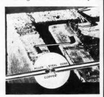
construction. The ties are made from high-strength Copperweld wire formed into a straight center stem with legs at both ends. The legs are projected at a 90-degree angle to the straight center portion. The tie has a modified "T" shape with all portions in the same plane.
