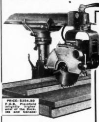
**Cutting** The smaller the blade required to make a given depth of cut, the greater its rim force. Walker-Turner Radial Saws use smaller blades than other types because their patented, geared motors get the shaft closer to the Walker-Turner work. The drawing at the right shows how this greater rim force is obtained, even with 50% less H.P. Write for RADIAL SAWS
