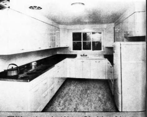
THIS kitchen contains a much-wanted feature—a U-shaped plan, to eliminate extra steps, with continuous working space. There is a ceiling ventilating fan over stove.
