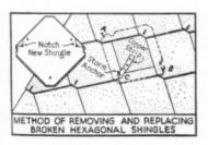
the nails will be cut off or drawn. Place a small piece of sheet copper over the storm anchor at "C" and nail it to the roof. Notch new shingle as shown, slip it in place and bend down the storm anchors.
