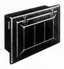
pressed steel .095 thick and arc welded at corners. The door is of 13 gauge pressed steel, ribbed for added strength and appearance. Hinge supports are of heavy stampings inserted through the
