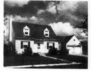
SYMMETRICALLY located dormers are often added to front elevation for ventilation in rooms added to second floor.
