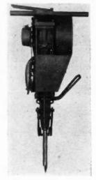
weighs 96 pounds, is arranged for easy operation by one man and uses moil points, narrow chisels, gads, wide chisels, frost wedges, clay spades, backfill tamping tools, asphalt cutters, sheathing drivers or ground rod driving tools, all with 11/8" x 6" shanks.
