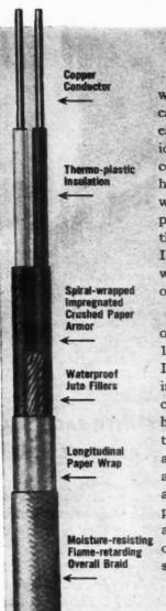
This new high quality, light weight, small diameter cable can be installed quickly and easily and will give long service. It is recommended for concealed and open work in homes and other building where non-metallic cable is permitted by local codes and the National Electrical Code It is approved by the Underwriters' for 60 degree to operation.
