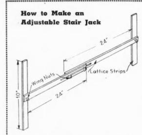
LAUREN DE WEESE, Moberly, Mo., in presenting this idea has the following to say: "This is a jack to cut in treads and risers in a stair. The ends are adjustable to the skirts and the center slot allows adjustment for length. I usually make it out of lattice with four wing bolts. two on the center and one on each end. The end of each piece of lattice shall be slotted about 6 or 8 inches long for wing nuts."
