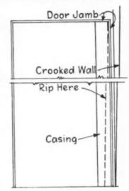
CECIL J. WALTERS, Newton, Kans. suggests this method of fitting a door or window casing adjoining a wall surface that is out of plumb:
