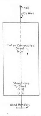
metal at points marked to rip directly over top of wire. Then stand on sheet at loose end of wire with feet close to the wire and at end of sheet. Pull up on handle about three feet high, then step back to repeat the pull until it has cut its way through the metal. With a little care the cut edges can be made as smooth as the factory edges."
