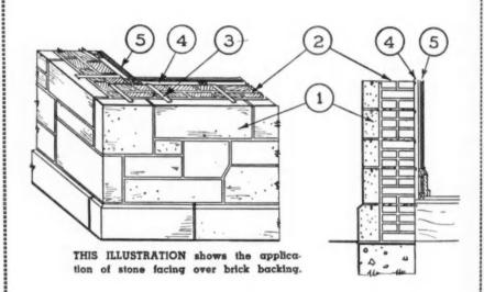
AS shown in the illustrations above, limestone is now cut in such a manner that it can be laid up as a veneer over a backed-up wall. It now can be used in moderately priced homes as a facing over the sheathing of a frame building, in exactly the same way as brick, stucco, or frame is used. Stone masons or brick layers lay it up in the wall. No setting drawings are necessary. Construction is as rapid as with other materials.
