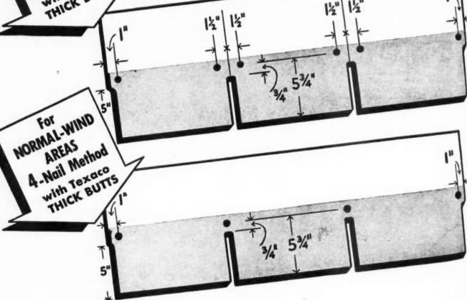
WARNING! Do not nail any higher than shown. Nailing in these positions increases resistance to lifting and tearing. It also keeps the nails in the thick butt portion.
