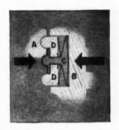
The new design of the meeting rail overcomes the problem of weather-stripping between two window sections!
