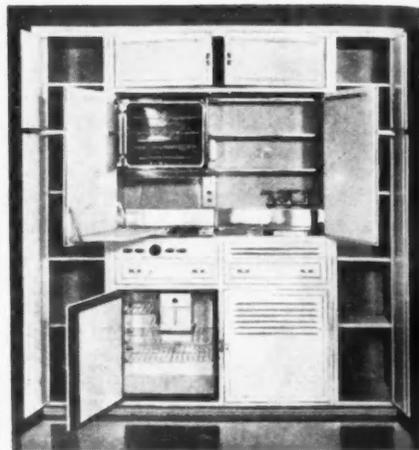
The model illustrated is the No. 700 gas kitchen unit, deluxe. It consists of a four-burner gas oven and broiler, and a 2.5 cubic foot capacity electric refrigerator. The basic unit is 46 in. wide, 22¼ in. deep and 81½ in. high. The side cabinets are 14 in. and are shipped separately to be added to the basic unit provided space is available. The sink and drain is manufactured from one piece of 18 gauge Monel metal with a satin finish. The exterior finish of the cabinet is a light gray.
