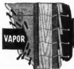
Insulite Lok-Joint Lath, with asphalt barrier against the studs, retards vapor travel. And Insulite sheathing, being permeable to vapor, permits what little vapor that escapes the barrier to pass toward the outside.
